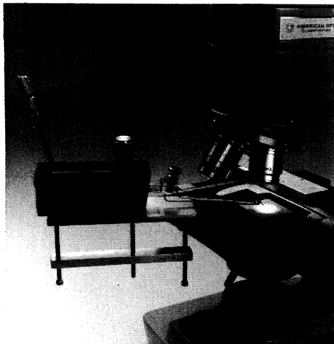
Fig. 19. Micromanipulator attached to a laboratory microscope. The manipulator allows precise control of the tungsten needle which is used to pick up particles for analysis.
