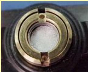
Small cup filled with powder in sample holder with spacer above cup
