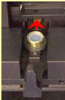
4. Place the sample holder on the sample insertion platform and slide it into the PAC 300 as far as it will go.
