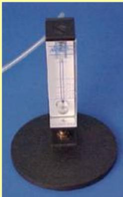
2. Use a length of 1/4-inch inner diameter plastic tubing to connect your helium gas source to the flowmeter inlet (bottom connector).
