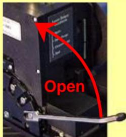
5. Set the sample chamber lever to Seal.
